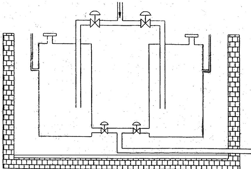
Figure I. Typical design of biomedical radioactive waste tank system.
