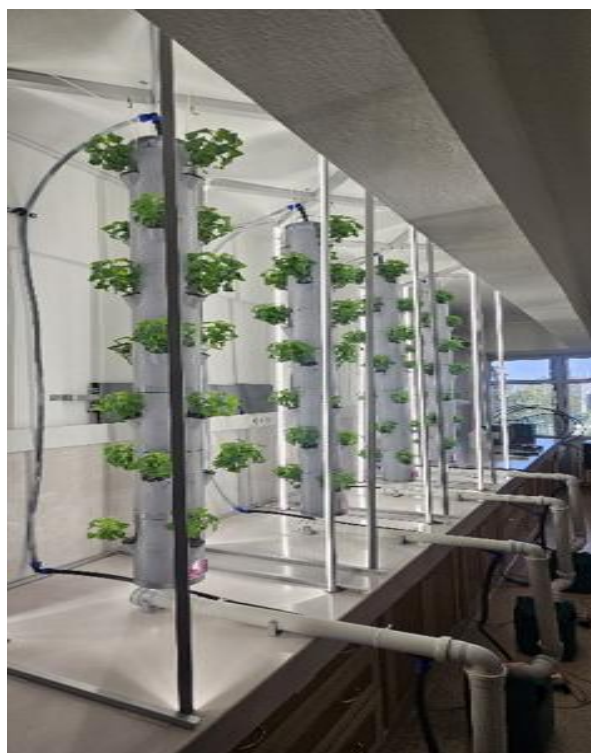
Figure 1. General view of the experimental setup (tower system and independent reservoirs).
