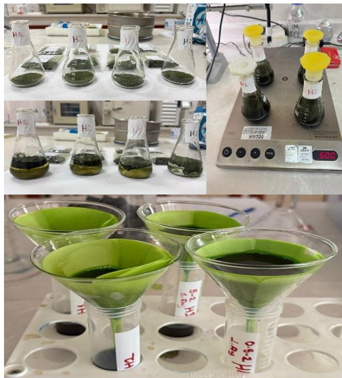
Figure 2. Extraction and filtration steps. (a) Extraction stage; (b) Filtration stage
