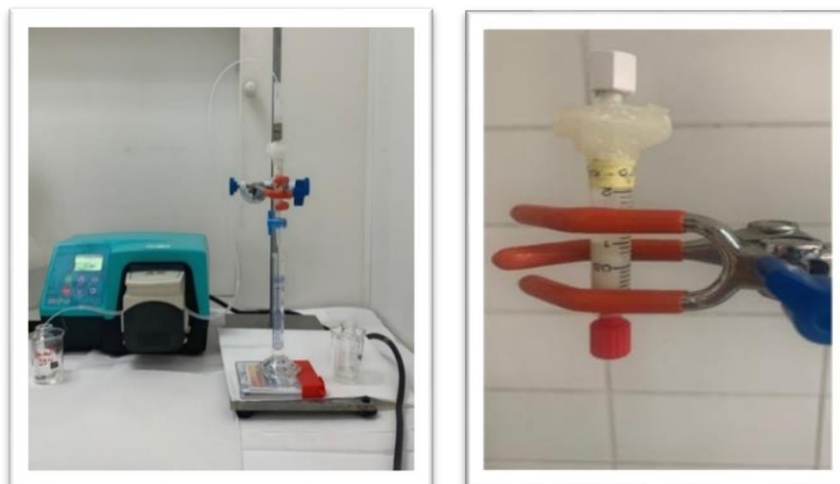
Fig.2. Experimental setup in order to determine the breakthrough of Ge from column
