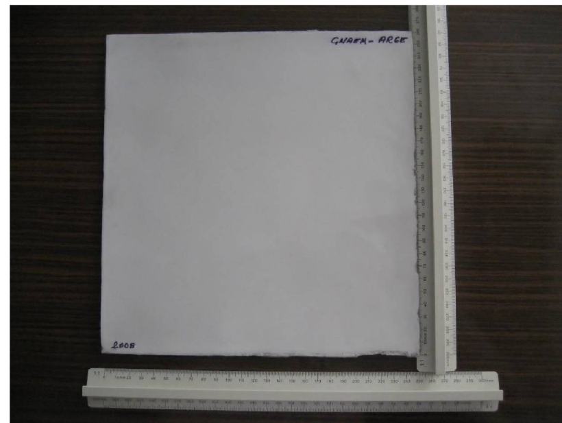
Scintillation Screen (27.5 cmx27.5cm with thickness 2.55 cm)
