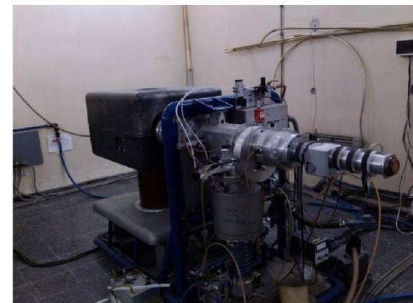
Sames J-15 Low Energy Ion Accelerator (Max. 150 kV)
