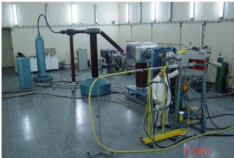
Sames T-400 Low Energy Ion Accelerator (Max 400 kV)
