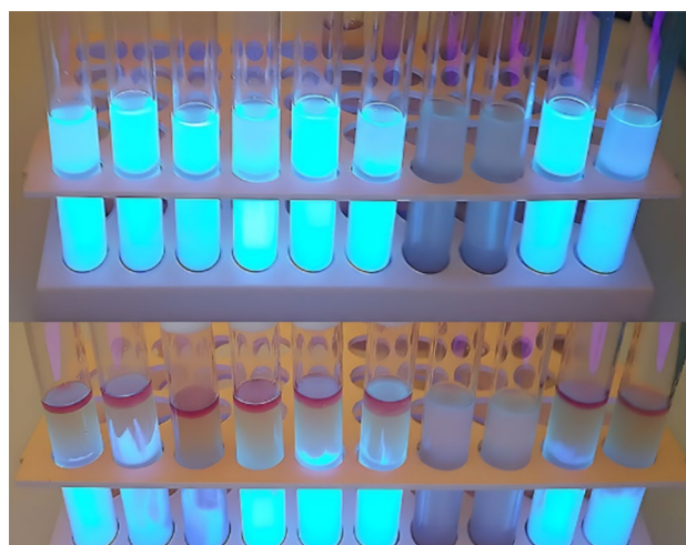
Fig. 1 Gas production, blue fluorescence, and indole ring formation tests for coliform and E. coli , obtained from LST broth medium supplemented with MUG
