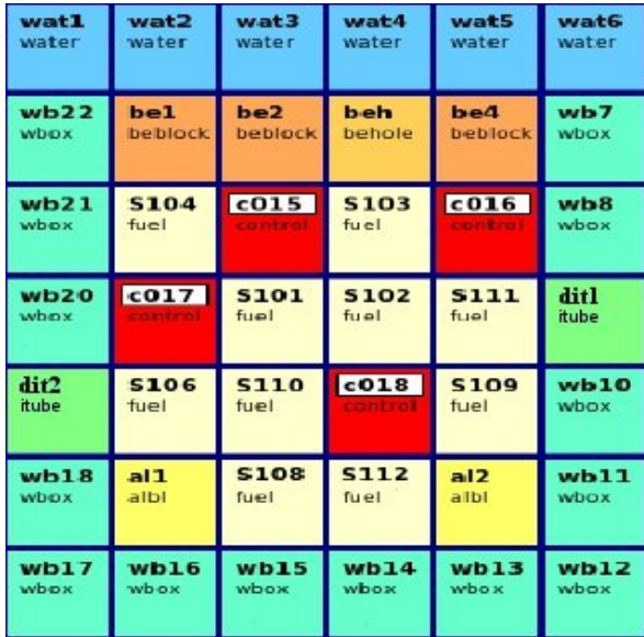
Fig. 2 Beginning of second core cycle configuration of TR-2
